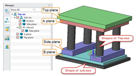
Figure 3. An assembly case1
