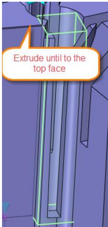
Figure110 Extrude sketch until to the top face
