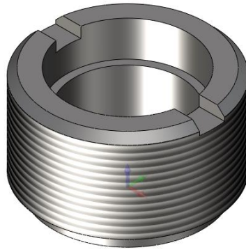
Figure 195 The Shim Compressor
